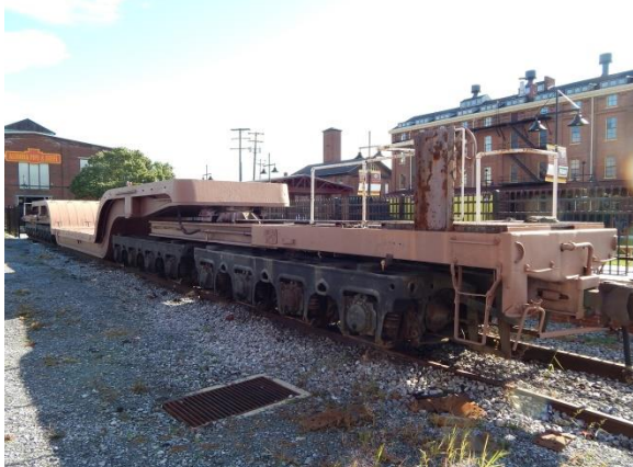
Pennsylvania Class FD2 16 axle depressed center flat car #47245 built in 1952 at the Altoona shops.
