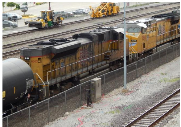
Westbound UP freight in Union Station passing a work crew on the siding. Mid-train units include GP40X #9002 and AC4460CW #7318.
