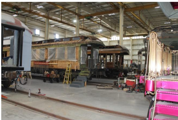
Restoration of wooden truss-rod coaches on the shop floor (photo by John Mezera).
