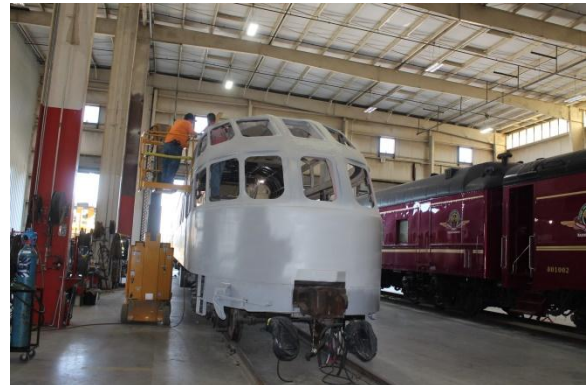
New window glass installation on former Hiawatha observation car (photo by John Mezera).
