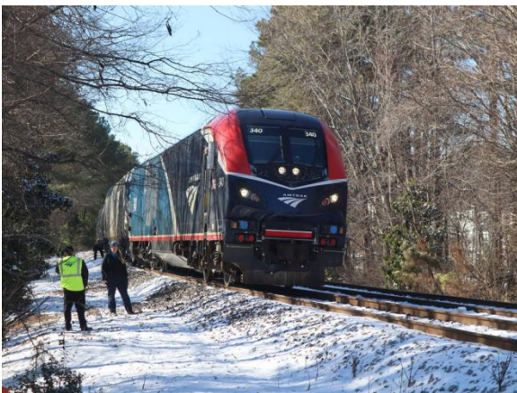
Uh Oh, Amtrak's Floridian is having some issues. One of the axles on lead ALC-42 340 fouled up. The trailing P42 not only had to push the lead engine to a nearby siding, but also had to pull the train all the way to Chicago on its own. On the bright side, the Charger received some love from the mayor of Apex on Facebook (1/22/25).
