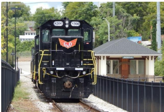
Knoxville & Holston River Railroad No. 8200 in Knoxville, TN. This is a National Railway Equipment rebuild of a GE 4L U-boat. Gulf & Ohio Railways is the holding company for K&HR and Three Rivers Rambler.
