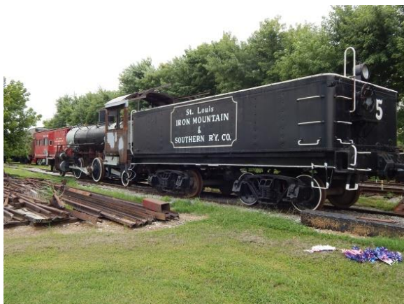
Restoration project 2-4-2 "Columbian" built by H. K. Porter, Inc. as a tank engine in 1946 at St. Louis Iron Mountain & Southern Railroad in Jackson, MO.
