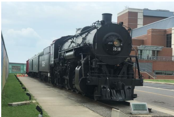
2-8-2 No. 1518 next to the flood walls in Paducah, KY. Built by Lima in 1923, No. 1518 was the last active Illinois Central steam engine.
