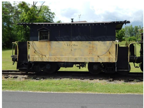
LC&M caboose No. 5 was built from a converted iron ore car in 1946
