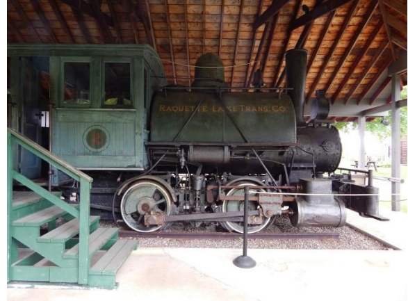
Marion River Carry Railway Porter 0-4-0 built in 1904. The entire railway was 1320 yards long and ceased operation in 1929.
