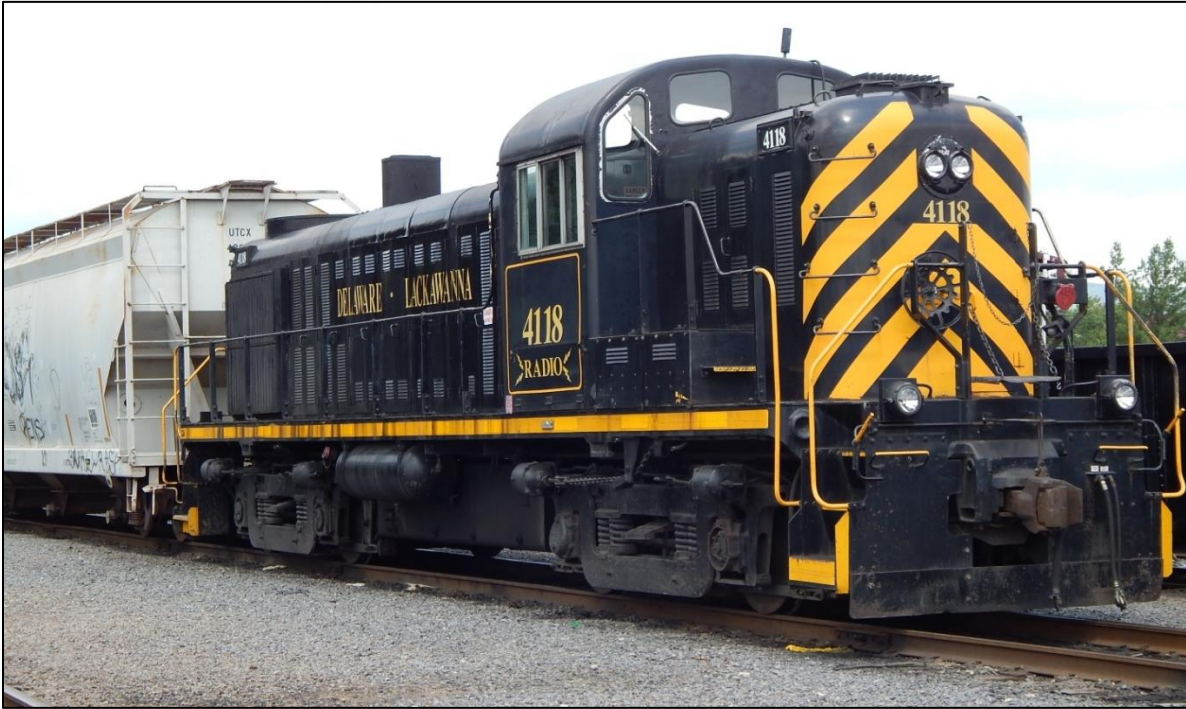
Delaware, Lackawanna, and Western Alco RS3 Number 4118 - note "RADIO" on the cab. There was a day when radio communication was the newest and best way to run a railroad.
