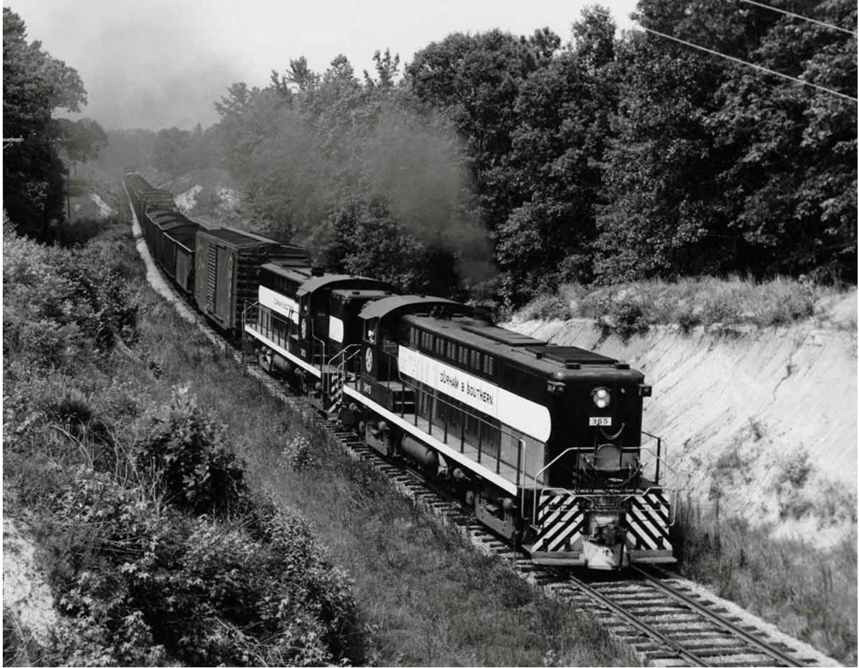
D&S 365 and 362, an example of the Baldwin DRS 4-4-15 locomotives Curt Tillotson Jr. photo
